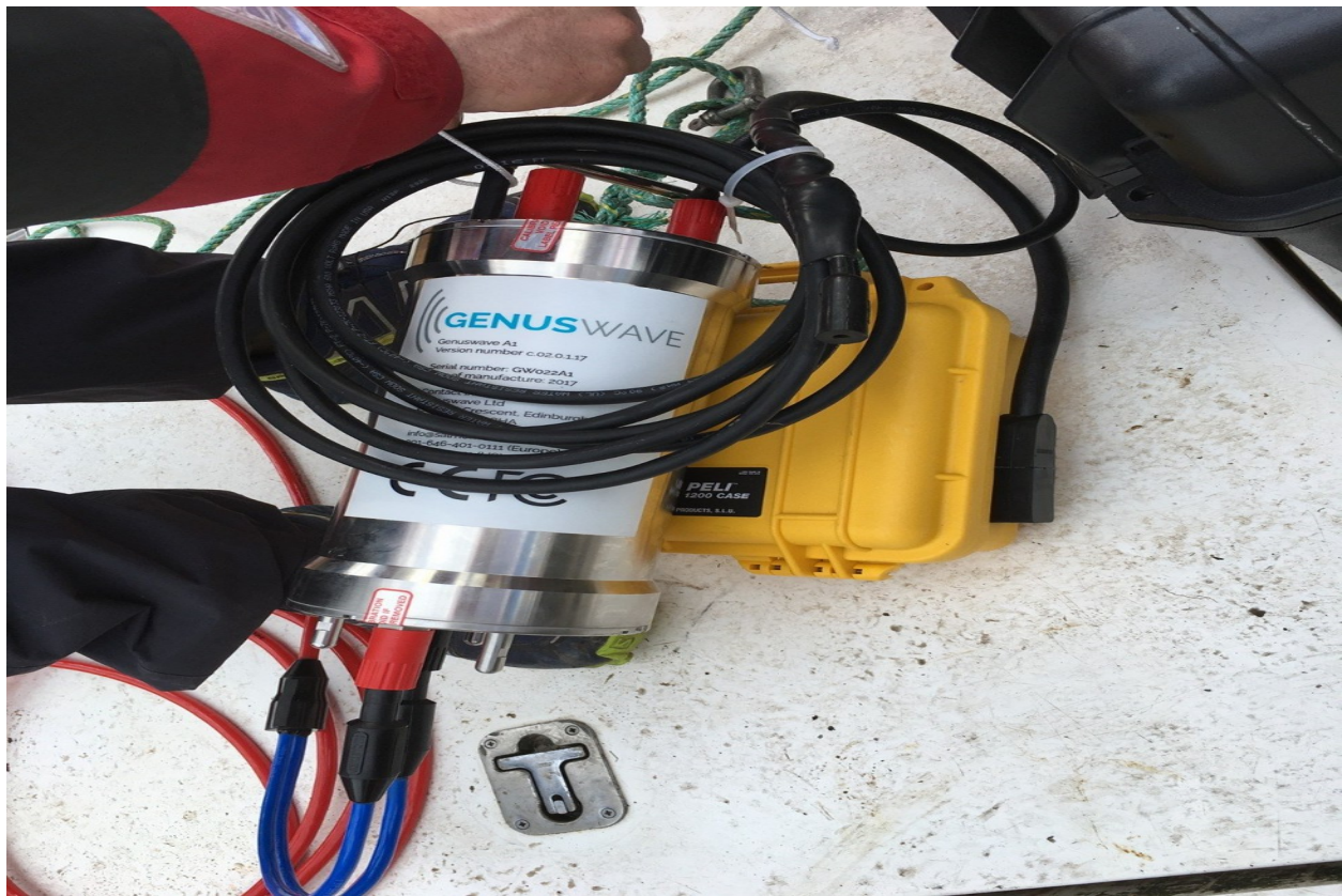
A Genuswave A1 unit being prepared for deployment, alongside its Peli 1200 transit case. The technology that reopened the freshwater intervention question — short, sharp non-impulsive signals that trigger the seal's startle reflex without habituation.
